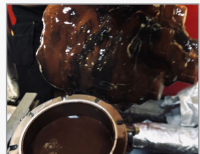
X-POT6 magnet grate with iron and biofilm
