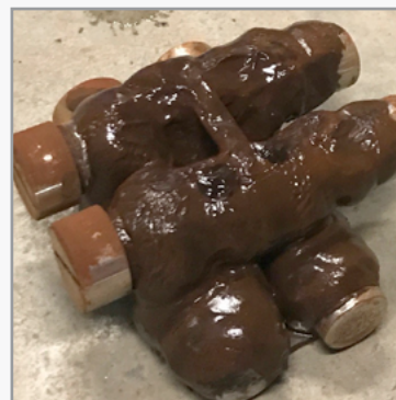
X-POT magnet grate capturing magnetite combined with biofilm.
